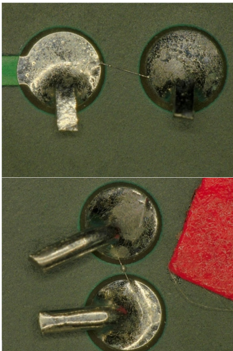
Figure 24: FeSn 2 IMC Phase Shorting Defect
